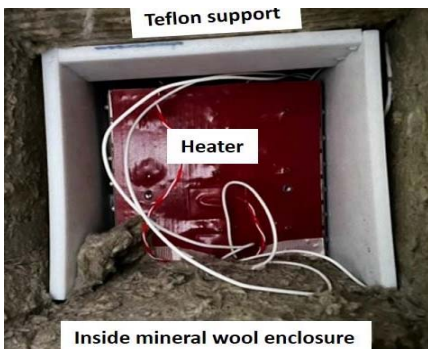
Front view of supermodule with attached heater pad
