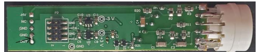
Mindy soldered ~800 50-V capacitors between signal and ground on divider base
