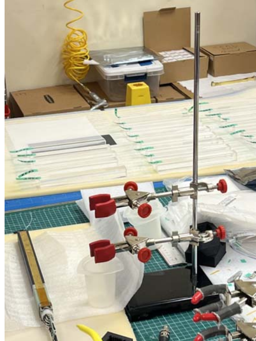
Crystals are cleaned and soaked in alcohol to remove glue holding light guide in place
