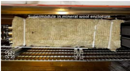
Insulated supermodule in oven. Industrial hygiene tested emissions to approve week-long tests
