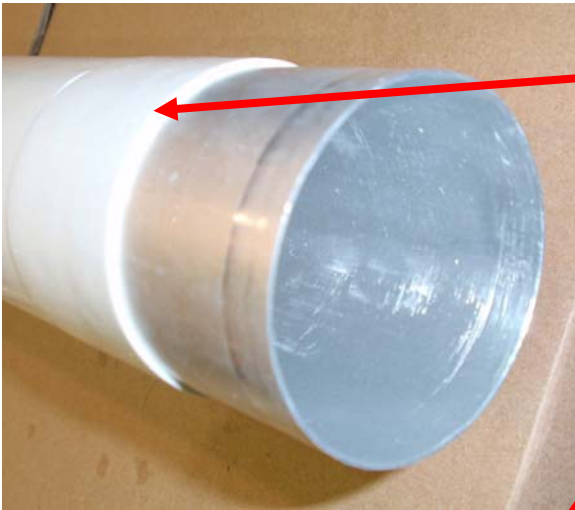
Beampipe wrapped with 1-mm aerogel
